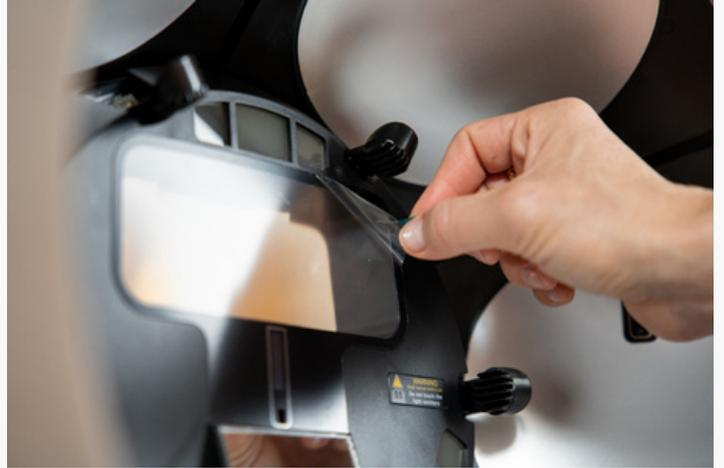
6. Move the iPad towards the back of Observ. Hook the visor in the top openings and tilt the visor to attach to the bottom of the device. Slide down the visor. When you hear a click, the visor is secured correctly.
